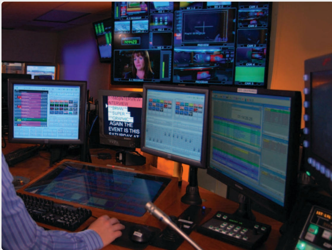
GRAY CONTROL ROOM LAYOUT. Using the Ross OverDrive Automation system, graphics are triggered in the newscast. Ross sends commands to the Media sequencer to trigger the needed graphics. The Director never sees a Trio playlist
